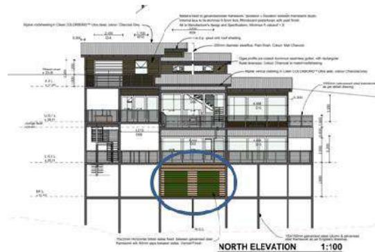
Figure 10: North elevation view which highlights the basement level storage of the water tanks by the blue circle (DEM TECH, 2020)
