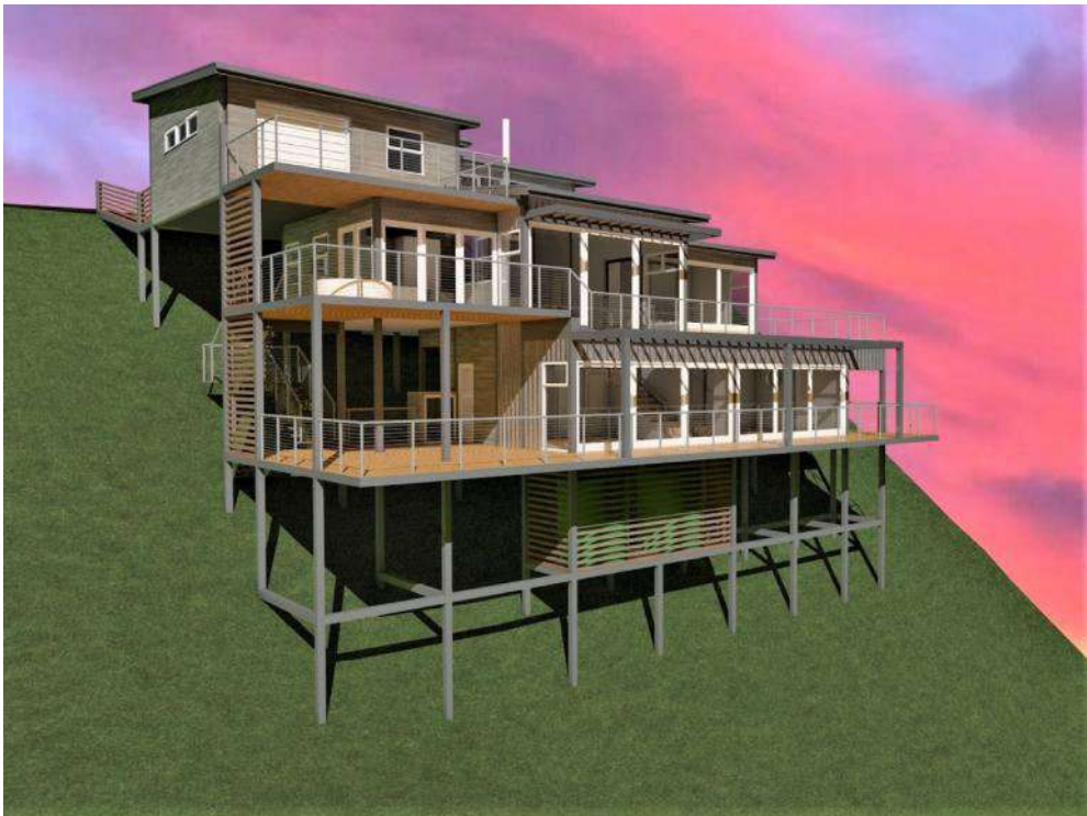
Figure 2: 3D Visual representation of the proposed dwelling - as can see from the image, the proposed dwelling will be on columns and will consist of various levels to limit the footprint area covered by the dwelling (DEM TECH, 2020)
