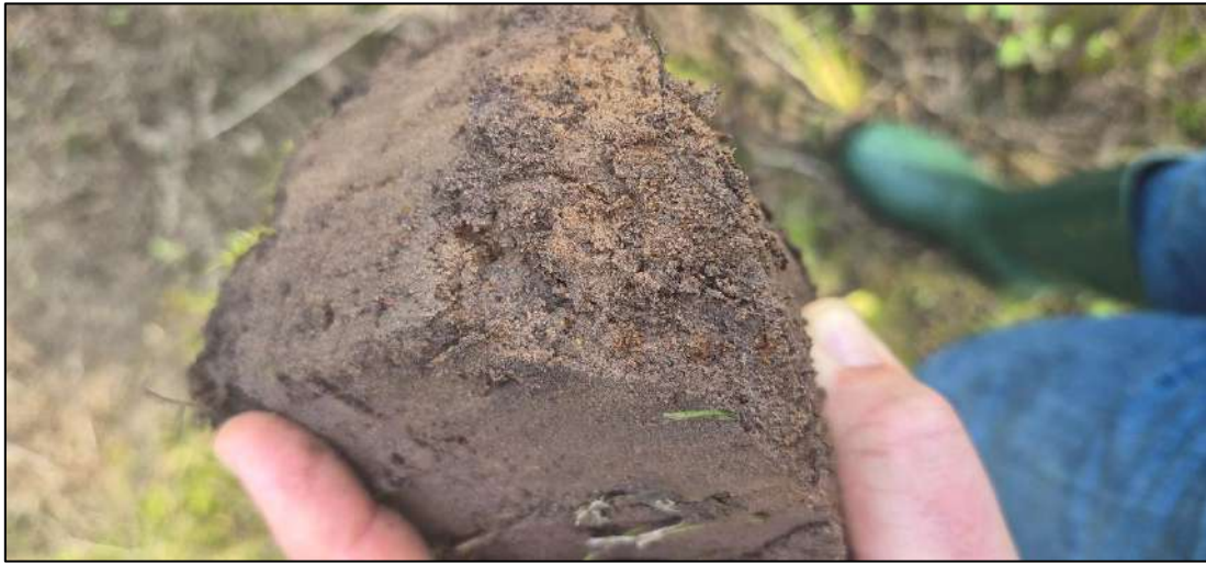
Plate 5: Photograph of a soil auger core from HGM 28 showing the presence of mottles despite the area being heavily farmed and soil historically disturbed.
