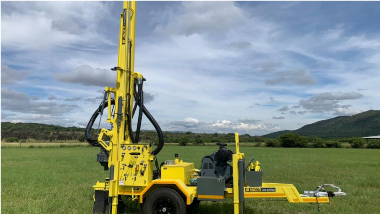
Figure 5 Example of trailer mounted rigging
