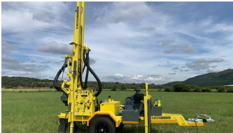
Figure 5 Example of trailer mounted rigging
