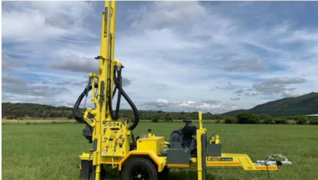
Figure 5 Example of trailer mounted rigging
