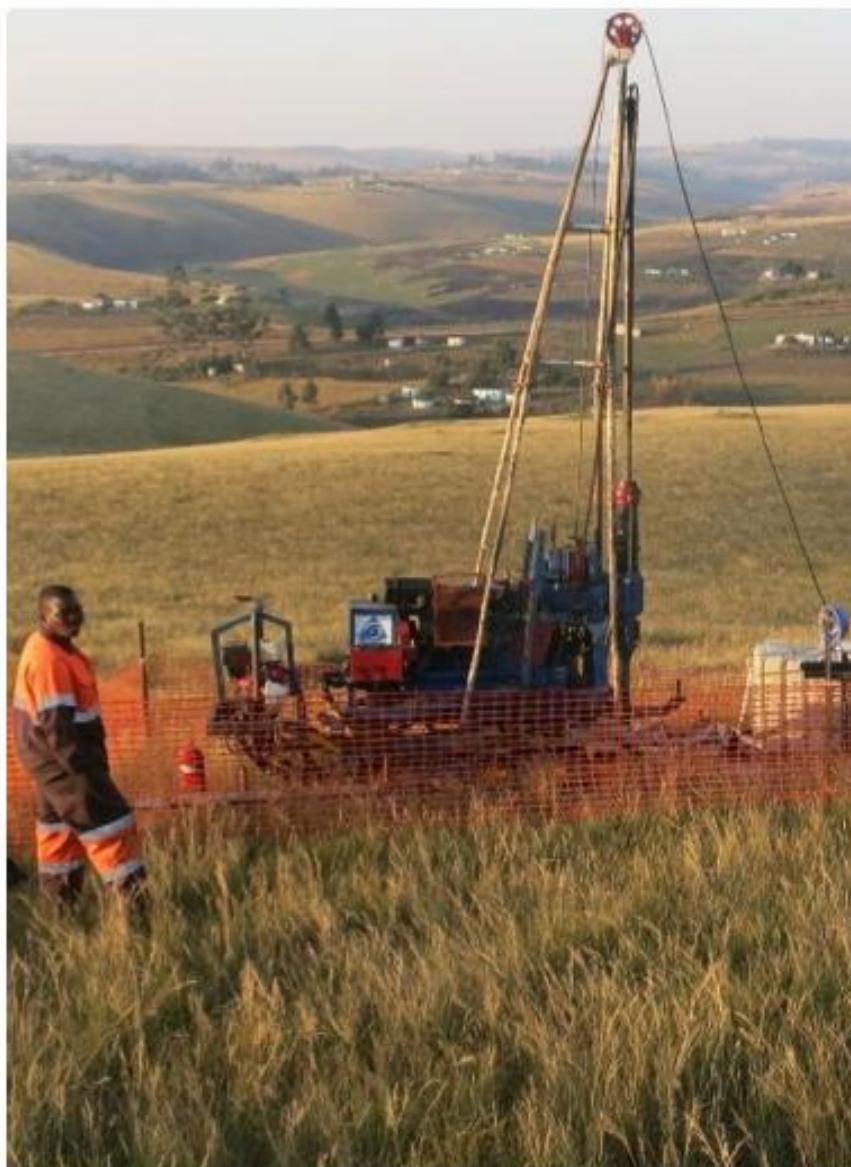
Figure 4 Example of core drill set up
