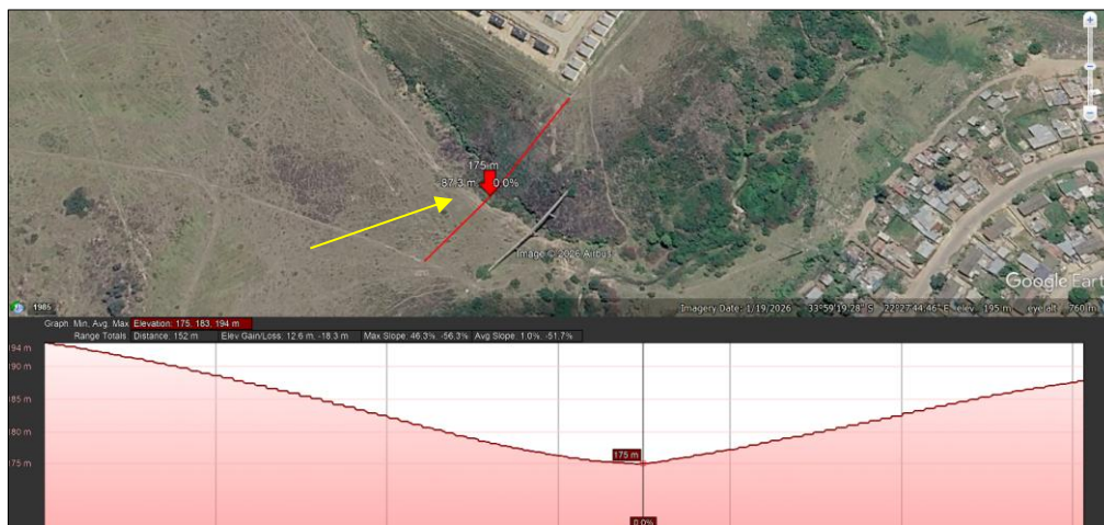
Figure 19. Google satellite image of Area A indicating the elevation profile (red line) across the valley with more dense vegetation and a steeper slope on the north-eastern side. Access here should be from the south-western slope (yellow arrow).
