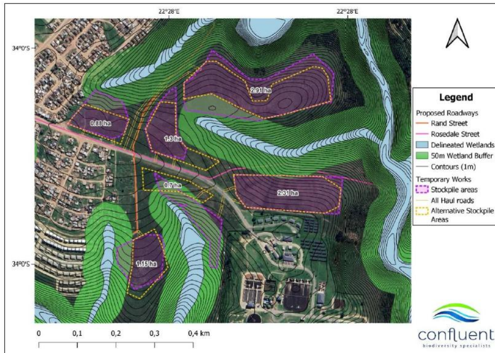
Figure 16. Proposed alternative stockpiling areas in relation to 50m wetland buffers and 1m contours.
