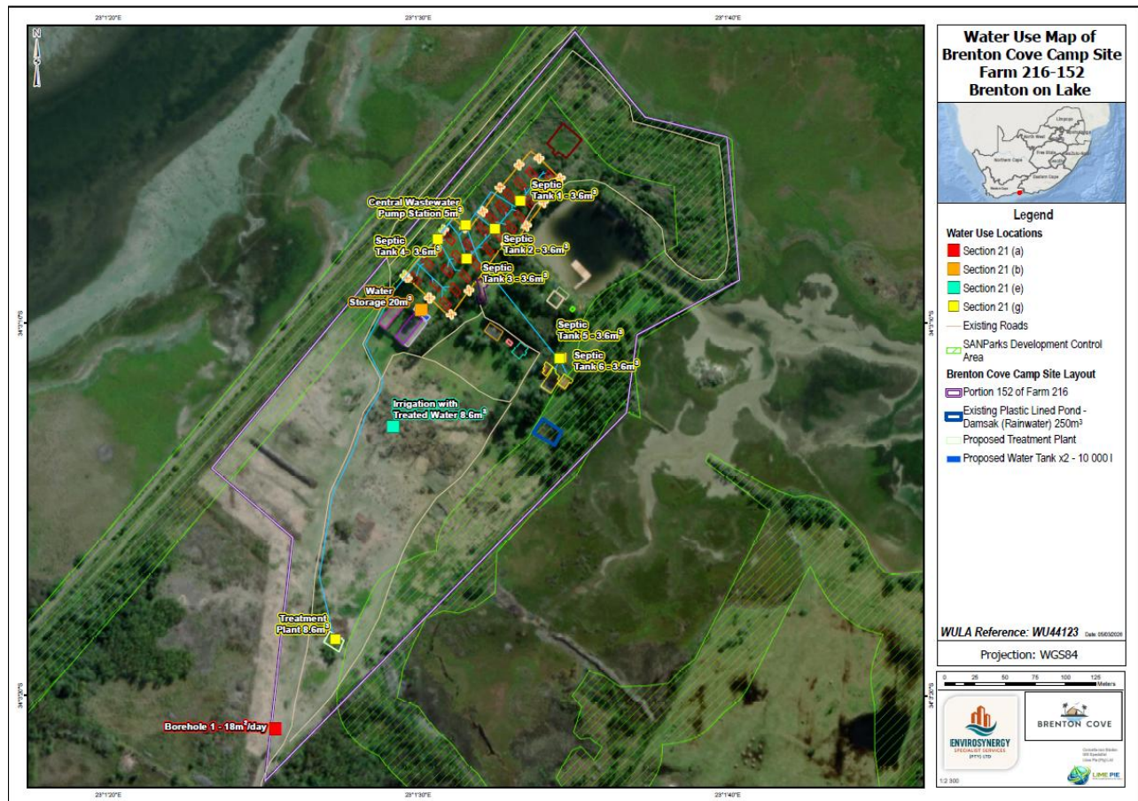
Figure 32 WULA site layout showing water uses (EnviroSynergy, 2026).
