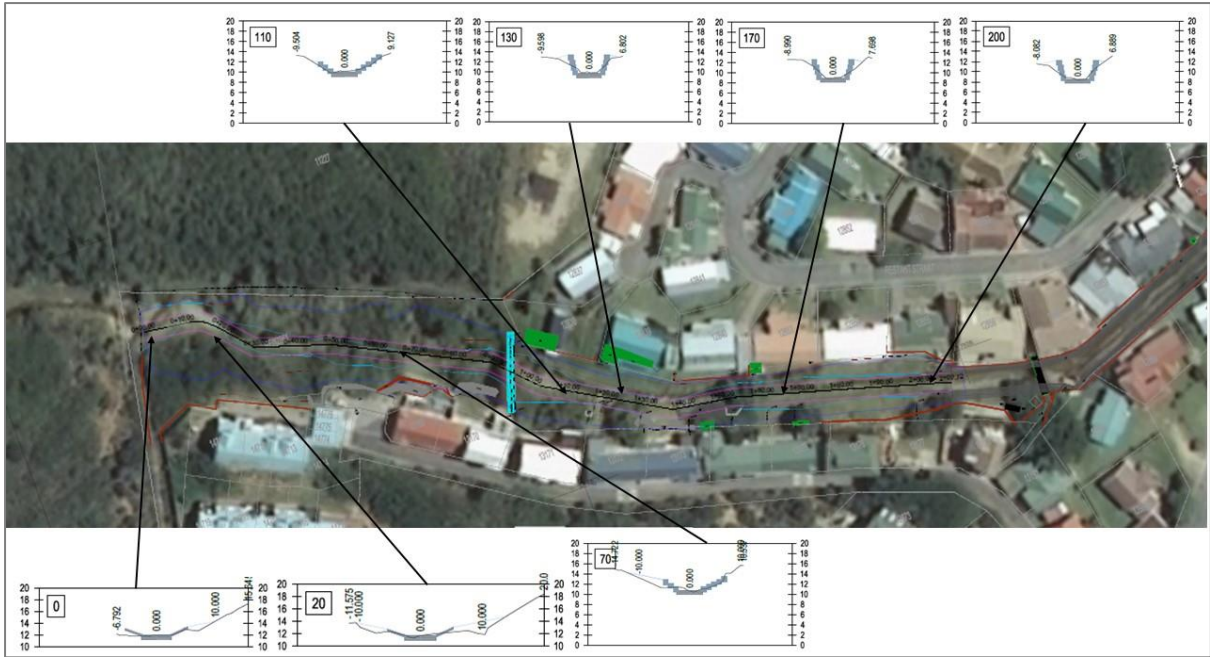
Figure 1. Simplified layout plan showing proposed cross-sectional bank and bed stabilisation (Modified from Appendix 1).
